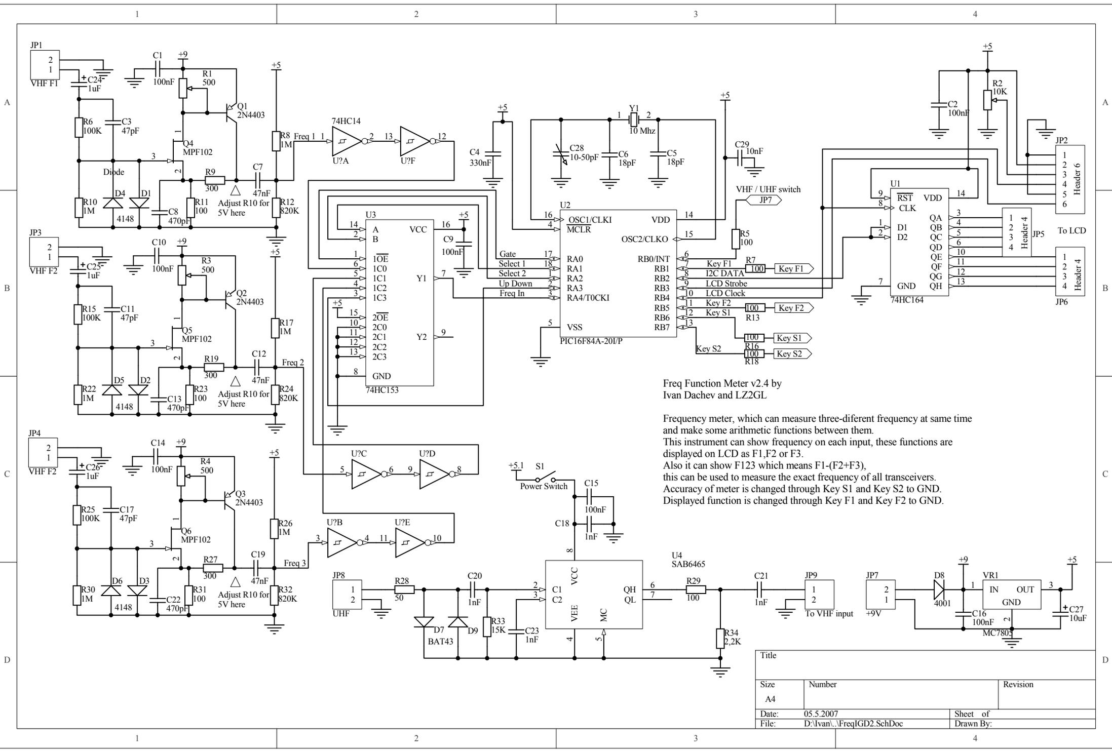
Freq Function Meter v2.4 by Ivan Dachev and LZ2GL
